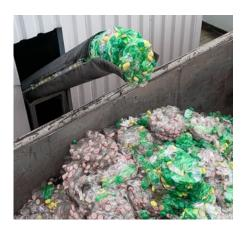
Flexible discharge due to increased discharge height and individual discharge length
